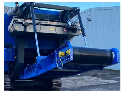
Overband magnet over the main belt
